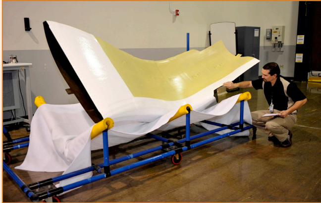
Figure B15. Northrop Grumman employee inspecting air duct from TAI. 27
