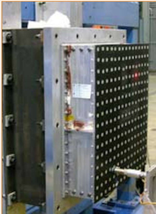
Figure B16. Composite Skin with SynCore center structure for F-35 inlet duct. 29
