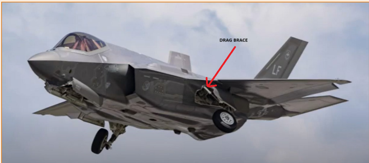
Figure B9. F-35 Drag Brace, Shown as a White Piston-Cylinder. 16
